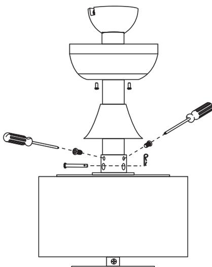
1. Thread the suspender through the suspended clock and coupling cover .
