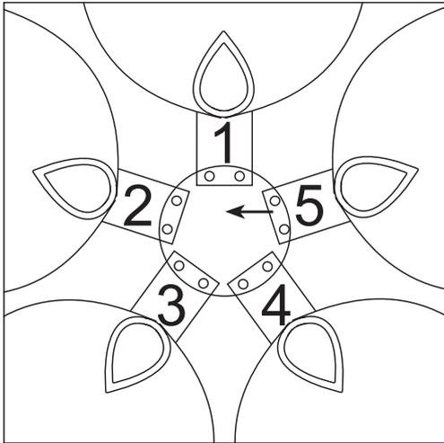
Put the clip in the center of a blade. Turn on the fan and, if the rolling persists, put the clip in another blade until the roll is reduced. It will be the blade that will need the counterweight.
